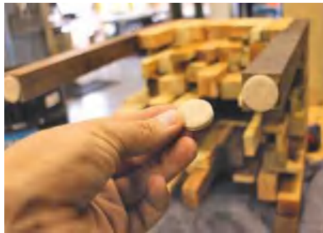
▲ Pic.7 Adding felt pads to the bottoms of the legs protects the project and your floor
